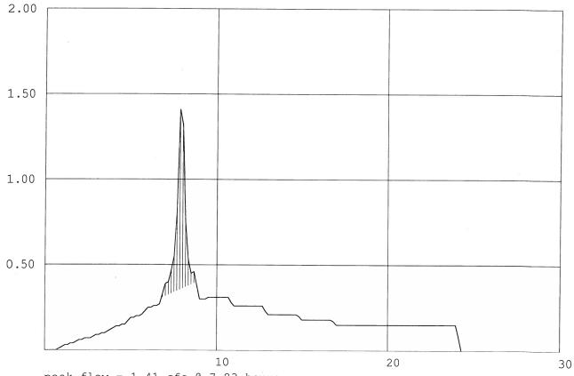
peak flow = 1.41 cfs @ 7.83 hours volume = 18,492 cu.ft. detention volume = 2,184 c.f. to limit flow to 0.40 cfs FEQURED
